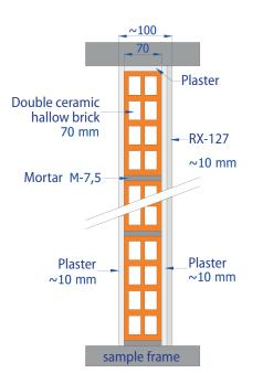
THE TESTED SECTION FOR THE DETERMINATION OF THE ACOUSTIC REDUCTION IMPROVEMENT CORRESPONDING TO **RX-127 RUALAIX ISOLXTREM**
