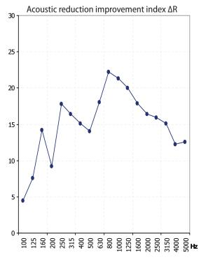
According to the UNE-EN ISO 10140-1:2011 standard, **RX-127 RUALAIX ISOLXTREM** applied in a thickness of 10 mm is capable of reducing the sound intensity by 3 dB from the transmitting enclosure to the receiving enclosure.
